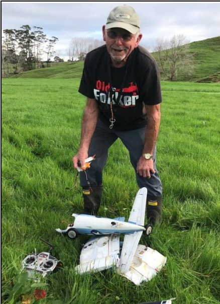
Baz's Corsair. He says his wings just folded up while inverted
